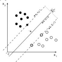
Maximum-margin hyper plane and margins for a SVM trained with samples from two classes. Samples on the margin are called the support vectors.
