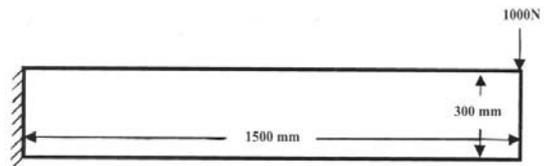
Fig. 5: Cantilever Beam
