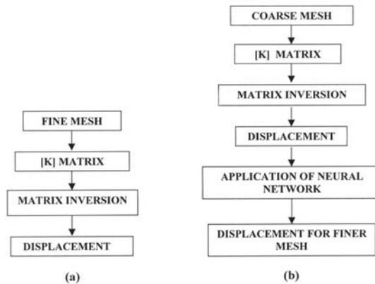
**Fig. 1: Flow diagrams (a) FEM (b) Neuro FEM**
