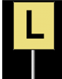
Fig. 5: Level crossing indicator
